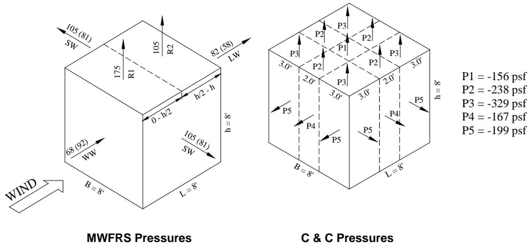
**Figure C10-1 Pressures on an 8' x 8' x 8' Shelter for Design Wind Speed of 250 mph**
