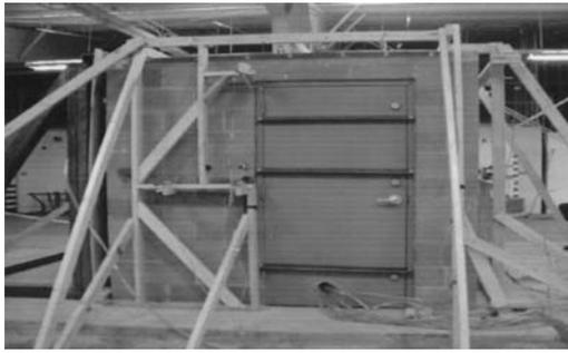
Fig. 9. Full-scale CMU specimen with instrument frame
