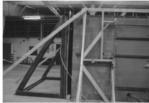
**Fig. 7.** External reaction frame
