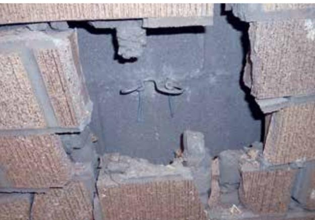
Figure 6. CMU surface behind missile strike on the Utility Unit Specimen 1 after testing.
