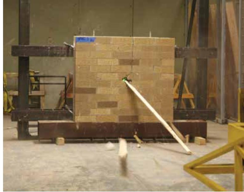
Figure 5. A first missile strike on Cavity Wall Specimen 1.
