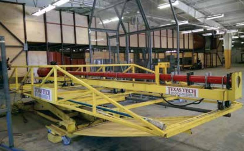
Figure 2. Tornado missile testing cannon.
